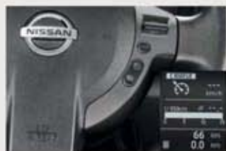
Driver adjustable speed limiter and cruise control
