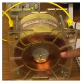
STOP PRELAB In the laboratory, an experimenter may easily control the current through a solenoid, and so it is desirable to determine the strength of the magnetic field inside the solenoid as a function of the current. Because of the high degree of symmetry in the ideal solenoid, Ampere's Law may be used to find the magnetic field inside the solenoid.
