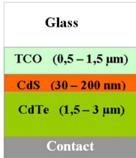
Fig. 20. Structure of CdTe thin film cell
