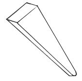
Everyday examples of wedges are an ax, nail, doorstop, horse plow, chisel, fork, and a saw. Scissors are two wedges working together to cut an object.
