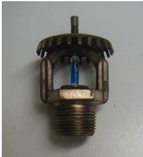
Large Drop 286°F Sprinkler Head
