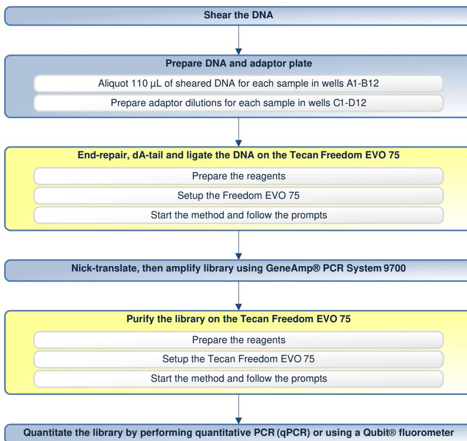
**Figure 1** Fragment library preparation workflow with the steps performed on the Freedom EVO® 75 displayed in yellow.
