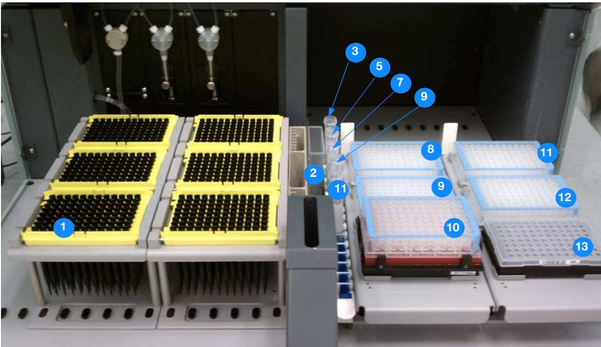
Figure 3 Layout of the worktable for Layout for SOLiD5500\_Frag\_Part 1
