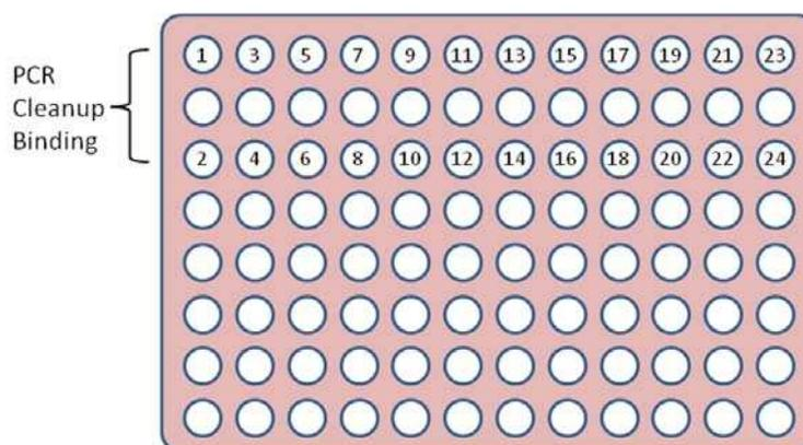
Figure 13 Eppendorf® 96/500-µL plate on VP771MM magnet at Grid 16, Site 3
