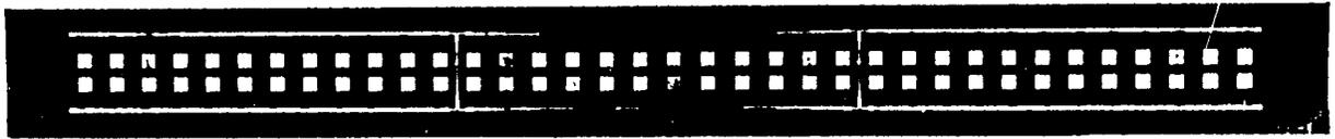
Figure 11. **Microstrip** array for aircraft **interferometric** radar remote sensing application.
