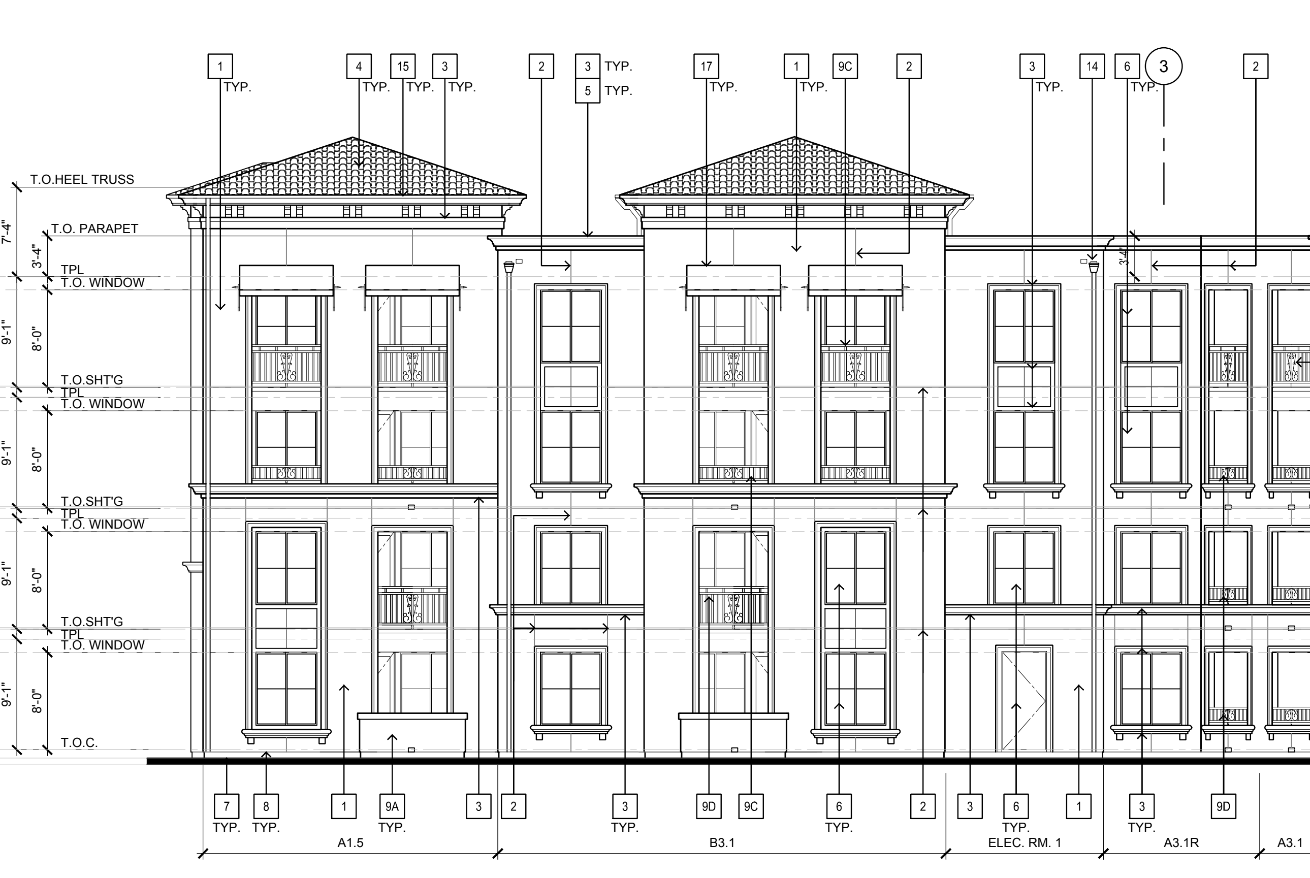
EXTERIOR ELEVATION - C
