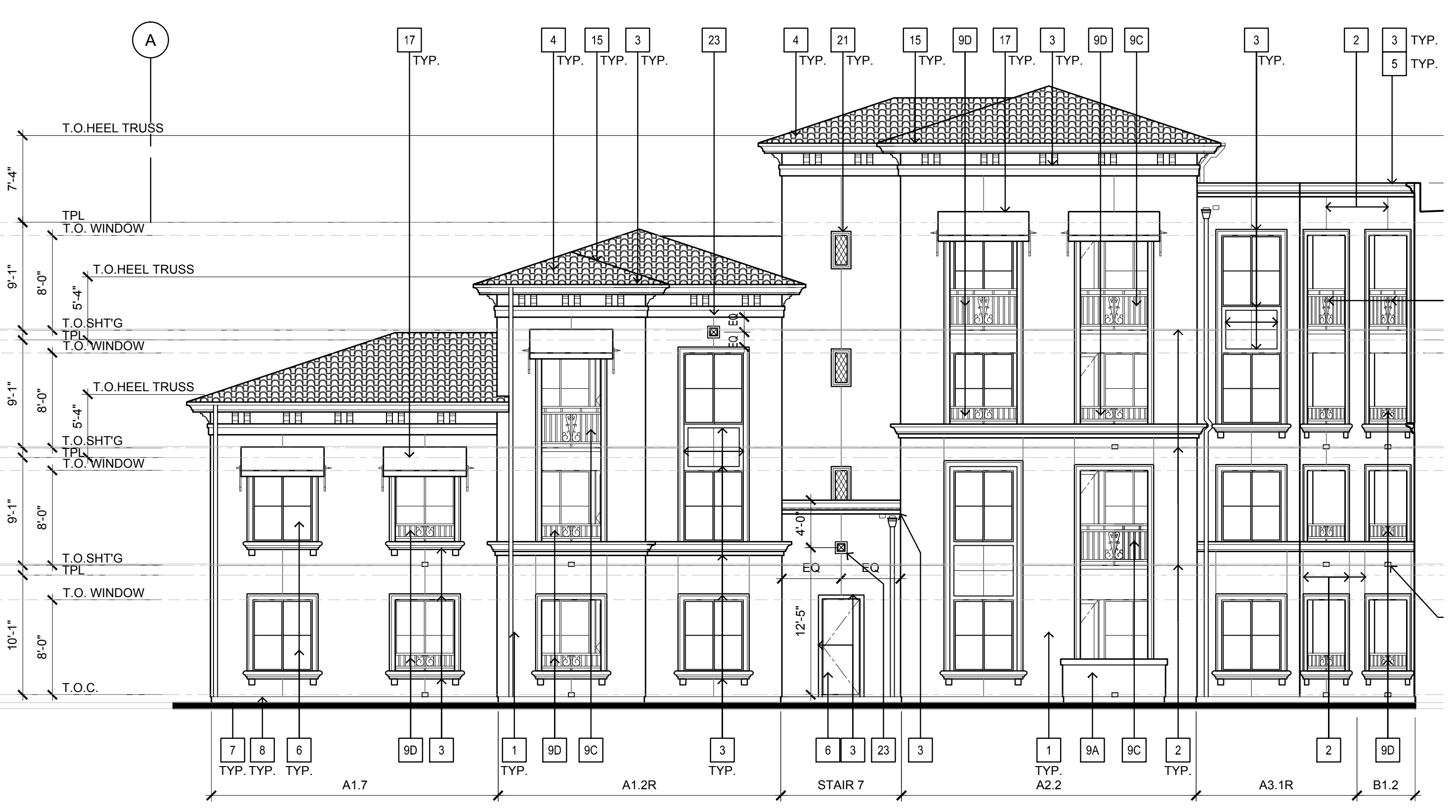
EXTERIOR ELEVATION - U 1/8" = 1'-0" U
