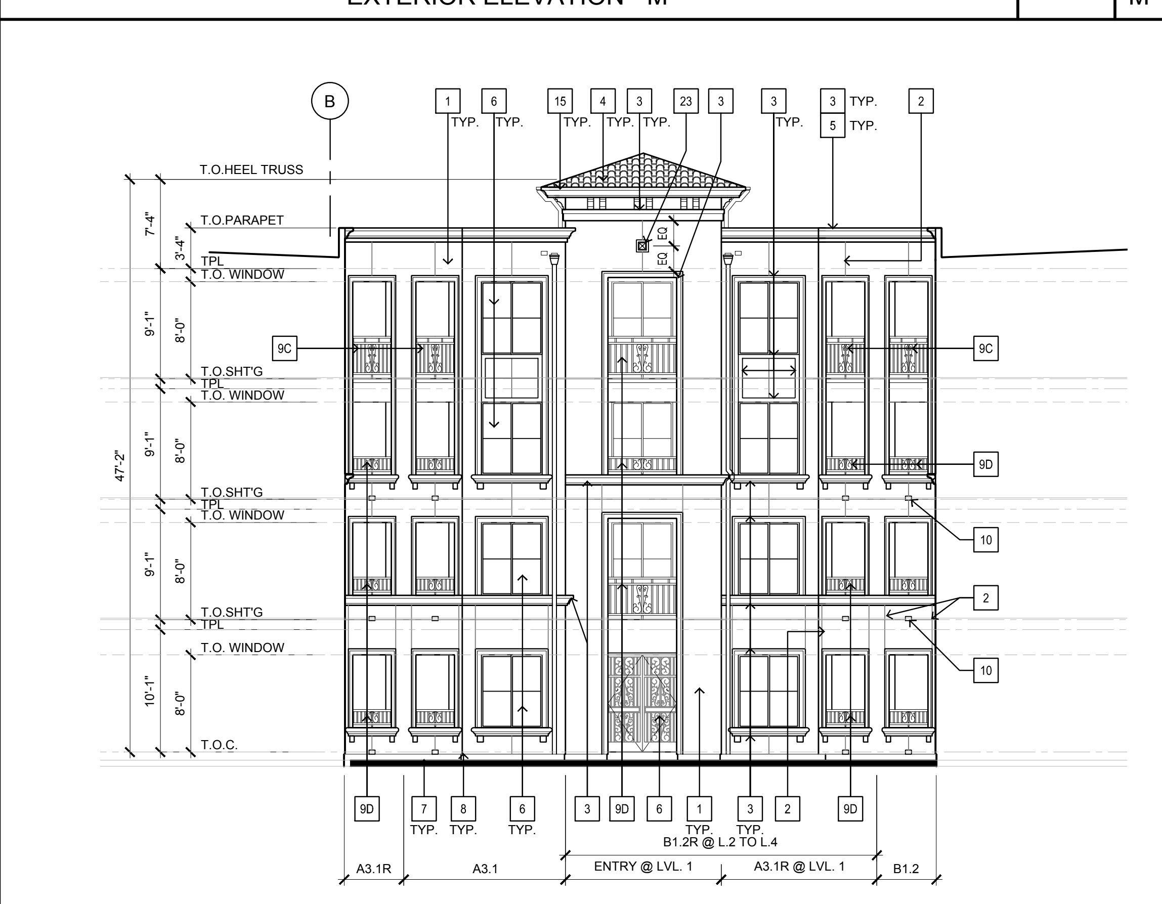
EXTERIOR ELEVATION - P
