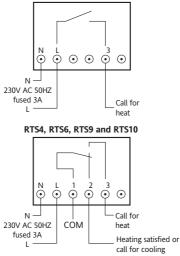
Note: Link between terminals L and 1 if mains voltage is required on the thermostat switch.
