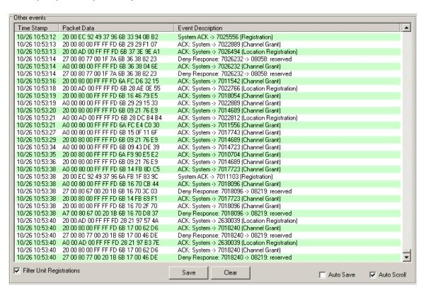
This screen includes the raw information from the control channel (Packet Data) and a description of what that data means. Since the majority of the entries on this screen tend to be unit registrations (Radios "logging on" to the radio system but not affiliating with a TalkGroup yet), there is an option to filter these packet types from this log.
