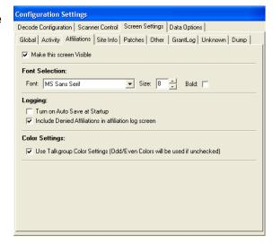
These options control logging of the information collected on this screen. The Turn on Auto Logging at Startup will turn on the automatic logging of affiliations when the program starts. The Include Denied Affiliations option controls the display of failed affiliations.
