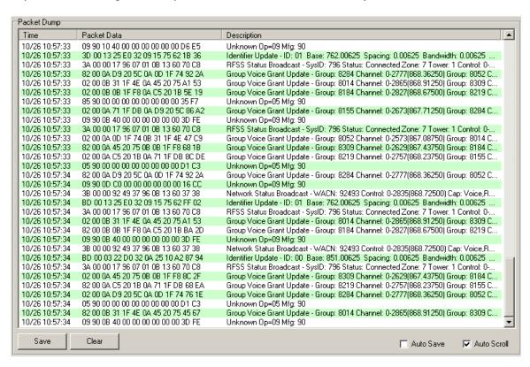
Note: This screen will store up to 10,000 lines of data, after which the first lines of data will be deleted. This has the effect of appearing to auto scroll even if the auto scroll checkbox is not checked.
