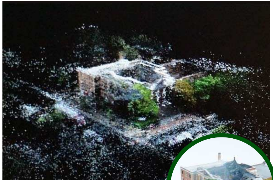
3D Point cloud data and resulting 3D model from the White Hall fire in Grand Junction Colorado Sept, 2011.
