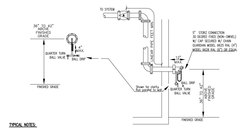
1)—ALL EXPOSED PIPING AND FITTINGS TO BE GALVANIZED WITH EXCEPTION OF STORZ CONNECTION
