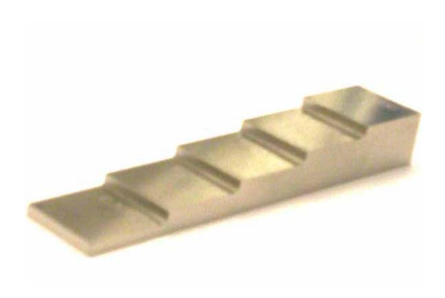
**Custom and Standard Test Blocks for Nondestructive Testing**
