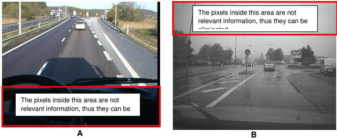
Figure 6: Example of filtering algorithm on cameras data.
