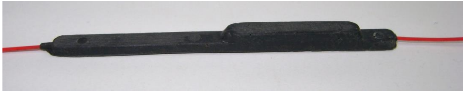
Figure 3 The fabricated sensor after the finishing process.
