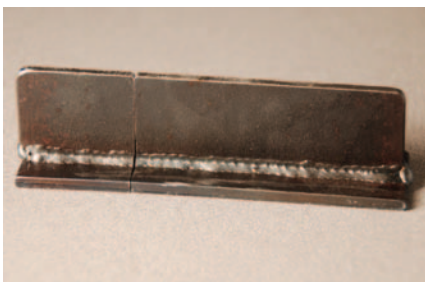
Fig. 1 — Sample of a visually acceptable single-pass fillet weld with poor fitup and lack of effective weld to one member. (See Fig. 2.)
