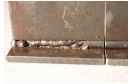
Fig. 6 — Sample of the backside view of a visually acceptable multipass fillet weld with poor fitup and a slugged and bridged root opening.
