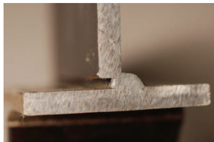
Fig. 2 — Sample cross section of a single-pass fillet weld with poor fitup. Notice the lack of effective weld to the vertical member.
