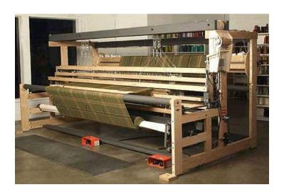
Note: 4-6' (1.2-1.8m) looms have all hardwood frames, 8' (2.4m) looms use powder coated steel for all crossmembers, and 10' (3m) looms and up are mostly powder coated steel.
