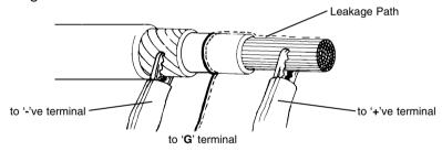
The guard terminal is at the same potential as the negative terminal. Since the leakage resistance is effectively in parallel with the resistance to be measured, the use of the guard causes the current flowing through surface leakage to be diverted from the measuring circuit. The instrument therefore reads the leakage of the insulator, ignoring leakage across its surface.
