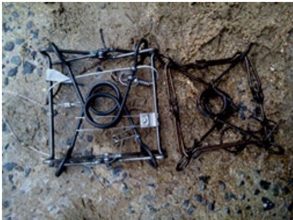
Image: 2 models of Body grip traps: Belisle Super X (top) and Duke (bottom), Albert Roura
