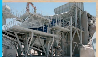
Scalping materials contaminated by clay are easily separated using a 'finger type roller grizzly' returning a high proportion of clean stone immediately back into the process. The benefit is increased yield from rock brought to the primary section, overall higher outputs, and reduced handling costs of generated waste materials.
