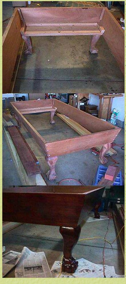
degree bevel at the end then layed one of my support boards in place and glued in the beveled sides. I placed my two 10 inch glue blocks at either end of the support boards and screwed them into place using 2 inch #10 screws. I did the same at the other end. I then layed in the rest of the left over Fir at the end. Cut them with 90 degree ends so they would fit tightly between the other two glue blocks. I ran 2 inch screws in both directions (down and out).
