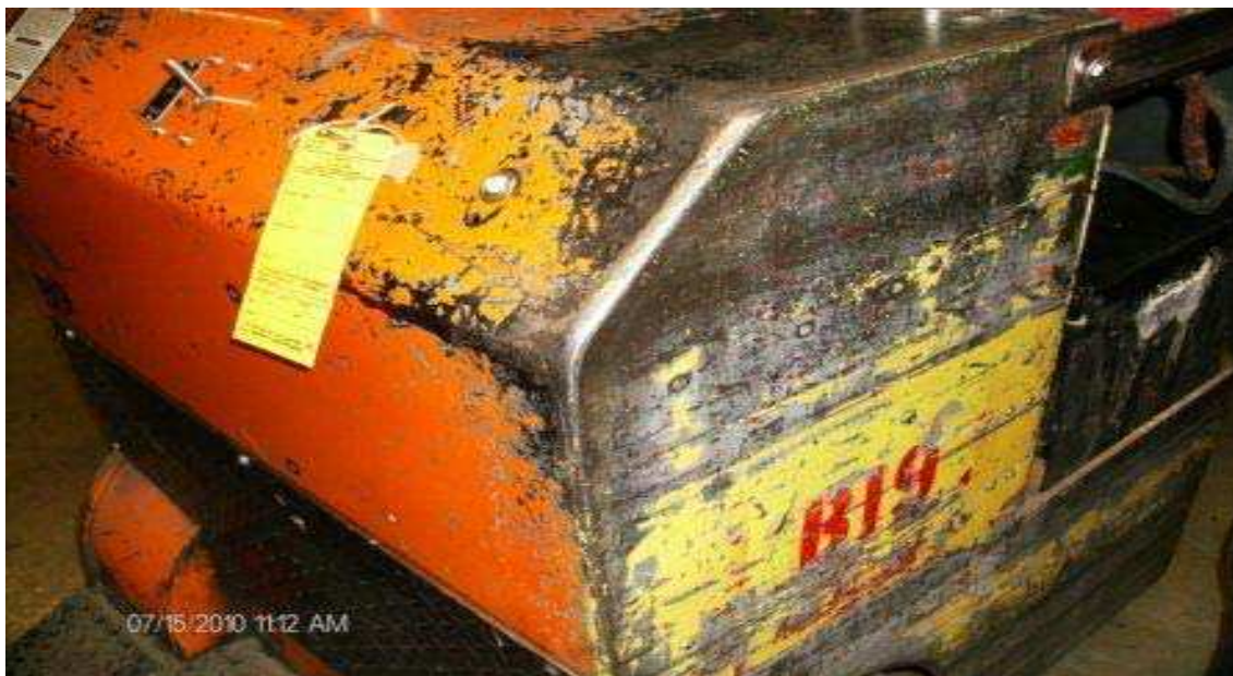
Illustration 3: The yellow tag on tow motor B-19 indicated that the brakes required repair on [REDACTED]
