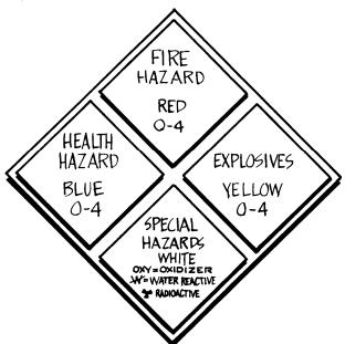
The NFPA 704M **labelling** system for hazardous materials was devised to provide at-a-glance information to response personnel on how a substance could be expected to react in the event of an emergency. RADIOACTIVE
