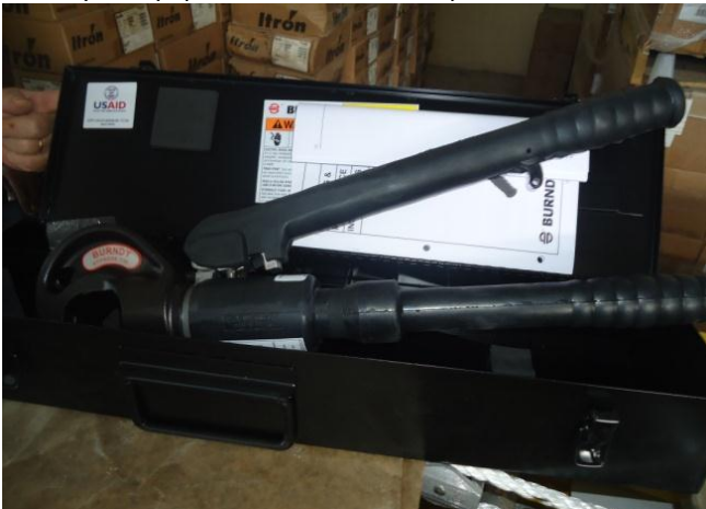
Shipment 3A - US0389-RFQ-2013-08 & US0389-RFQ-2013-09 - Commercial & Technical Tools Burndy Products, MD7-8 manual crimping tool
