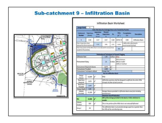
An Infiltration Basin is the selected practice to manage the runoff from the remaining areas and flows that are not fully reduced in other practices (sub-catchment 9 (blue shaded area)). The 'Infiltration Basin' worksheet is used to determine the reduction credit for this sub-catchment. Select 9 in the Catchment # drop down menu to import the sub-watershed design information.
