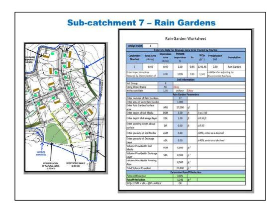
Rain Garden is the selected practice for sub-catchment 7 (bright green shaded area). The 'Rain Garden' worksheet is used to determine the reduction credit for this sub-catchment. Select "7" in the Catchment # drop down menu to import the design information.
