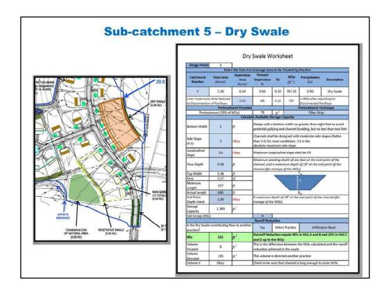
Dry Swale is the selected practice for sub-catchment 5 (orange shaded area). The 'Dry Swale' worksheet is used to determine the reduction credit for this sub-catchment. Select sub-catchment 5 in the Catchment drop down menu to import the design information for this sub-catchment.
