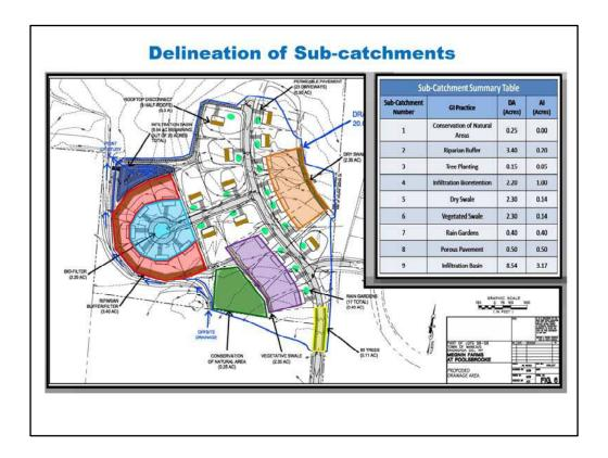
For this example, the site has been broken up into 9 sub-catchment areas. Below, is a summary of the 9 sub-catchments and the practice chosen for runoff reduction.
