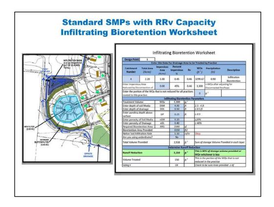
Note: An Infiltrating Bioretention is a form of bioretention without underdrains. It can only be used in areas where the soil infiltration rate is 0.50 in/hr or greater. If the soil infiltration rate is less that 0.50 in/hr or if underdrains are proposed, the 'Infiltrating Bioretention' worksheet is not appropriate and the designer should use the 'Bioretention' worksheet.
