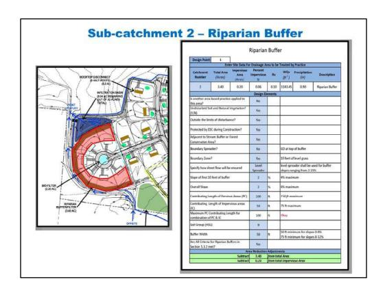
Riparian Buffer is the selected practice for sub-catchment 2 (red shaded area). The 'Riparian Buffer' worksheet is used to determine the area reduction credit for this sub-catchment. Select sub-catchment 2 in the drop down menu in the blue cell under catchment number to import the sub-catchment design information.
