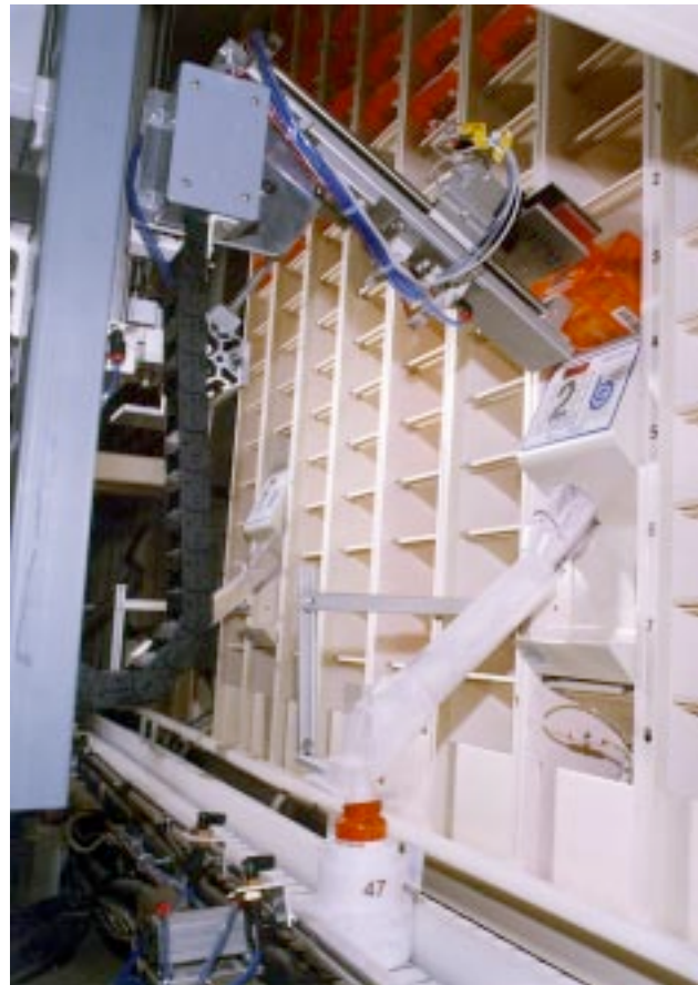
The robotic arm makes automatic placements on a counting device and the correct quantity is dispensed directly into the waiting bottle on the conveyor belt. The bottle then continues to the filling technician who completes the order.
