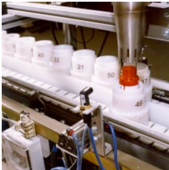
After the Pharmacy Baker 3000 assigns a barcode to a prescription, scans it, generates a label and drops a bottle into the automatic labeler, the bottle goes into a "puck" on the conveyor belt. Each numbered white puck has a unique microchip in it to aid in the tracking of the medication through the filling process.
