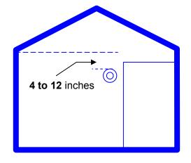
In areas with flat or sloped ceilings the top of the smoke detector must be located between 4 and 12 inches below the point where the sidewall and ceiling of the home intersect.
