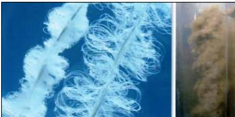
Clean BioCord material shown on the left. Biocord with accumulated Biofilm shown on the right
