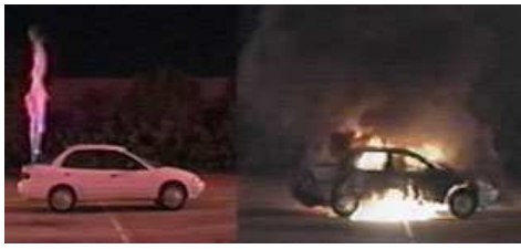
Hydrogen car (l), gasoline car (r). Photo from a video that compares fires from an intentionally ignited hydrogen tank release to a small gasoline fuel line leak. At the time of this photo (60 seconds after ignition), the hydrogen flame has begun to subside, while the gasoline fire is intensifying. After 100 seconds, all of the hydrogen was gone and the car's interior was undamaged. (The maximum temperature inside the back window was only 67°F!) The gasoline car continued to burn for several minutes and was completely destroyed. Photo/Text: Dr. Swain, University of Miami.
