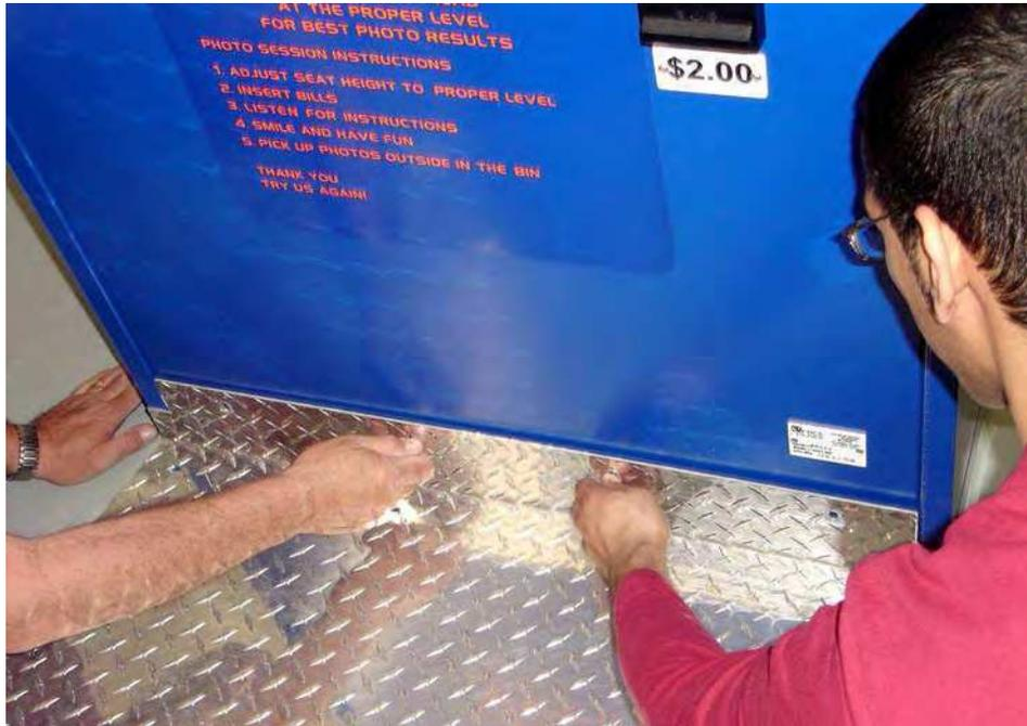
13. Using 2 people, carefully lift the Seat Unit top over the Seat Unit and Camera Unit.
