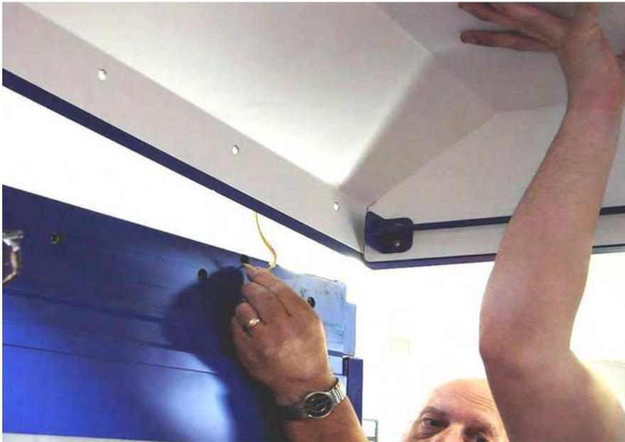
15. Set the Seat Unit Top down on the Seat Unit side first. The 2 short, white tabs on the bottom sides of the Seat Unit Top stay outside of the Seat Unit (visible if inside the booth). The long, white tab (found on the bottom of the Seat Unit Top) gets inserted into the Seat Unit.
