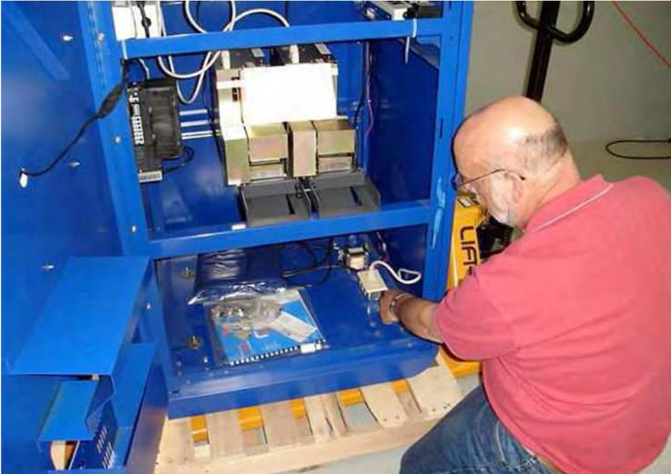
8. Push the Camera Unit to edge of the pallet. Carefully tilt over while someone pulls the pallet from underneath.
