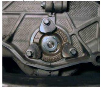
LN Engineering also offers an IMS Upgrade service where you send in your intermediate shaft and it is upgraded to a triple row bearing (with exception of MY06-08). Additionally, the main drive sprocket is pinned to prevent slippage of the drive gear, which is a known problem area.
