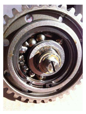
One thing is for sure; once you have experienced an IMS bearing failure, there is no turning back. A complete engine disassembly is required to replace the intermediate shaft and in most cases, complete rebuild or engine replacement is your only option.
