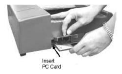
☐ 63. Insert the scanner key and turn it to the **OPEN/CLOSE POLL** position. It will take approximately two minutes for the scanner to load the election definition from the card into its operating system. The scanner will display "S-MODE" in the upper left corner of the LCD screen and the message "ELECTION CARD INSERTED, OPEN POLLS NOW?" DO NOT PRESS YES TO OPEN THE POLLS AT THIS TIME.
