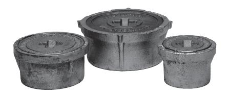
The Model W watertight flush fill caps screw onto the threaded end of fill and/ or sounding lines to provide full diameter access to the tank through a watertight terminal. The assembly consists of a rust-resistant, galvanized cast iron body, with a gasket sealed solid bronze cover for a waterproof seal.
