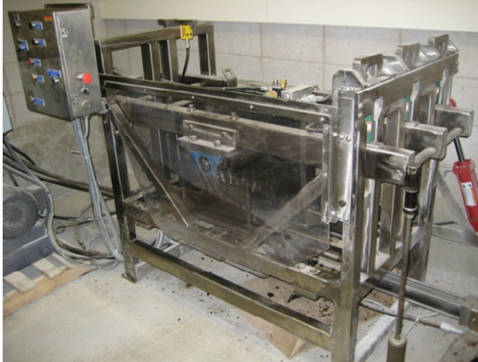
(a) Roller compactor
