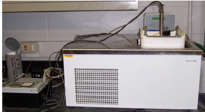
Figure 4. Test setup for CTE
