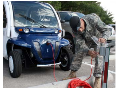
Figure 6-5. Spc. Dean Kalogris from Headquarters Company, Fort Bliss, Texas, charges the installation's command sergeant major's electric car using Level 1 charging equipment. Photo from Major Deanna Bague, U.S. Army, NREL/PIX 18634
