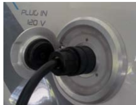
Figure 6-4. Level 1 plug-in hybrid electric vehicle charging port. Photo by Ted Sears, NREL/PIX 17342
