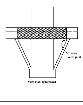
Piper Model PA 34-200T Seneca Wing Flap Control Cracks 2750
