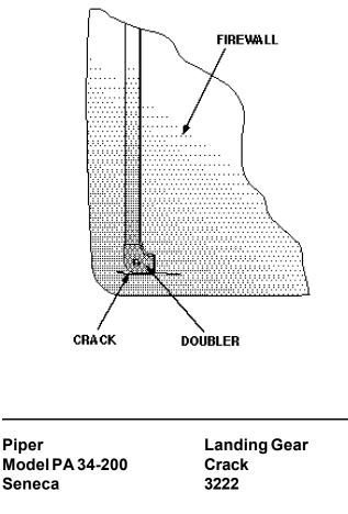
During an annual inspection, the nose landing gear trunnion was found cracked.
