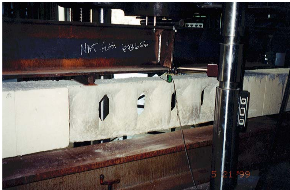
Figure 4 Steel I-Beam, Loading Points, and Deflectometer
