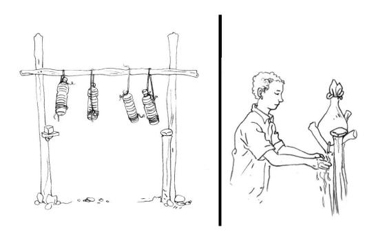
Handwashing stations can be very simple and still be effective. Using Tippy Taps made from bottles or gourds can also save water.
