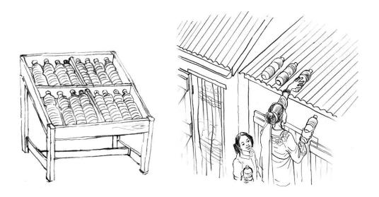
Solar disinfection (SODIS) with plastic PET bottle placed in the sun is an easy way for classes to make drinking water safe. Here is a a SODIS stand that parents built, and a teacher placing bottles of water on the class roof. After 6 hours in the sun, the water is safe to drink.
