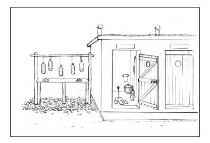
Latrines with a "Tippy Tap" handwashing station, made from empty plastic bottles. The handwashing station has a "soakaway" drainage area made with small stones to avoid puddles.
