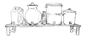
Drinking water can be safely stored in may different kinds of containers, as long as they are clean and well covered, and the water can be served without making the water dirty. These containers have spigots or taps that can be inserted into jerrycans and plastic buckets.
