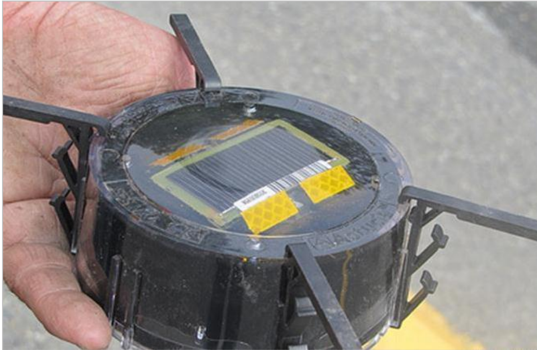
Figure 9 WSDOT solar reflector
