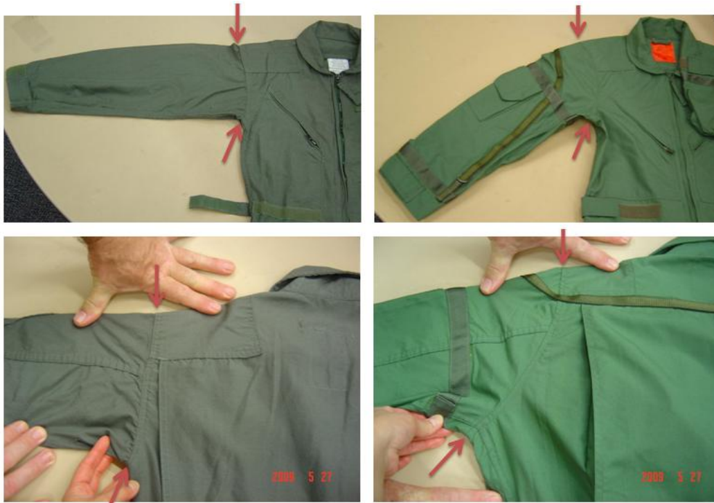
Figure 19. (a-d). Shape of the Scye seam comparison. a) Front view of 27P size 36S (Top left), b) Front view of RFDB size 2B (Top right), c) Back view of 27P size 36S (Bottom left), d) Back view of RFDB size 2B (Bottom right)
