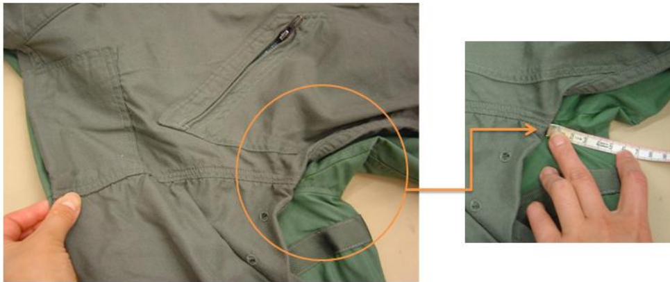
Figure 18. Scye ease comparison between 27P and RFDB (Top is 27P size 36S and bottom is RFDB size 2B, about 5cm difference)
