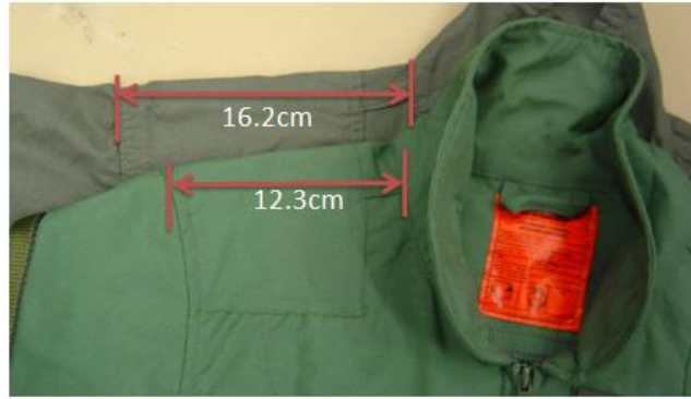
Figure 20. Shoulder area comparison between 27P (Bottom, 16.2cm) and RFDB (Top, 12.3cm) test flight suit (Aligned at the center line-Zipper)
