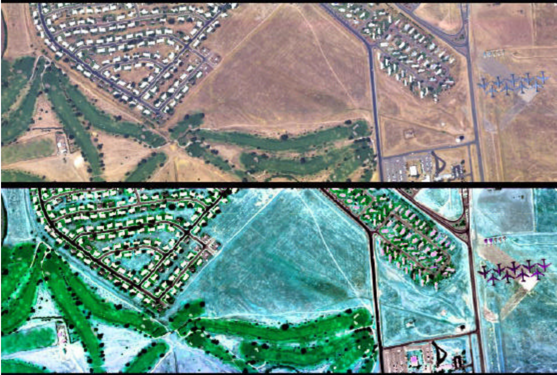
Figure 6.5. Davis-Monthan Air Force Base: A. Natural color, B. -30 -degree rotation of RGB Transformation via HSV colorspace operations.
