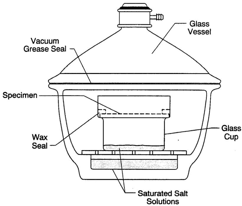
Fig. 3. Schematic illustrating experimental method.
