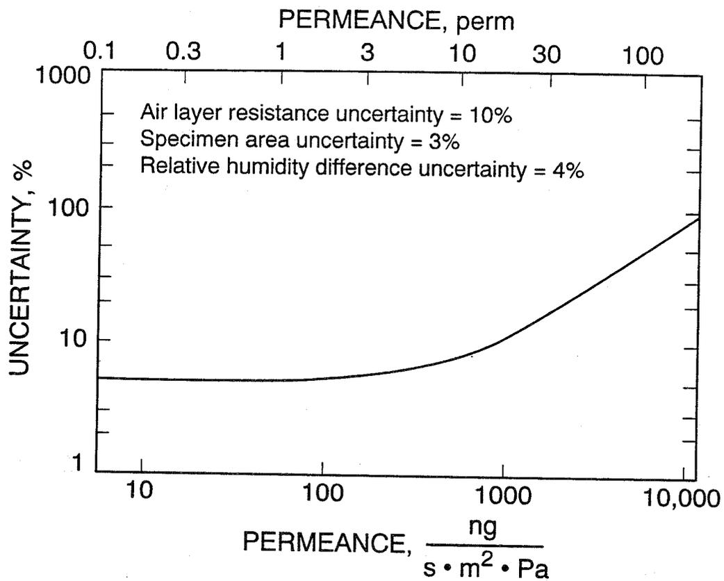
Fig. 12. Plot of uncertainty of permeability measurement versus specimen permeance.
