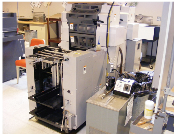
View of press from the feeder end with Royse recirculator to the right.
