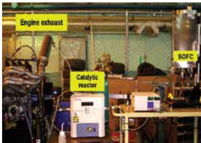
Fig. 3. Experimental setup used for the validation of the concept using exhaust from an internal combustion engine as feed.
