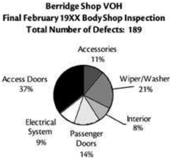
Figure 1. Percentage of Defect by Component, Berridge Shop
