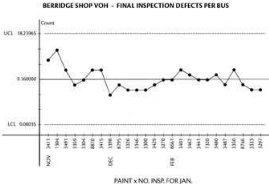
Figure 3. C-Chart Application from SEPTA's Paint Shop
