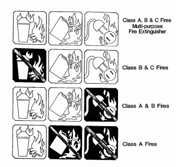
The symbols with the shaded background and the slash indicate that the extinguisher must not be used for that type of fire. The Certificate of Fitness holder must understand these symbols. Generally, there are clear operation instructions on the side of the fire extinguisher. The describe how to use the extinguisher in case of an emergency. An example of these instructions is shown below.
