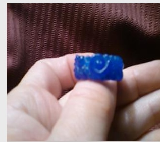
Medieval wax ring carved and ready for casting (back view)
