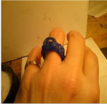
Medieval wax ring (gem) carved and ready for casting
