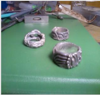
Contemporary band (foreground) cast and ready for polishing
