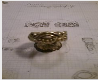
Medieval style ring cast and ready to clean (sketches of ring in background)
