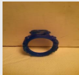
Medieval style wax ring (gem) carved and ready for casting
