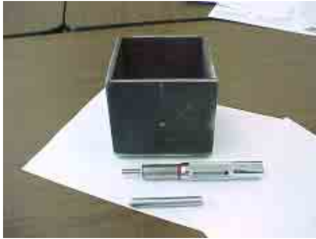
Figure 5.1: Workability box and penetrometer with adapter
