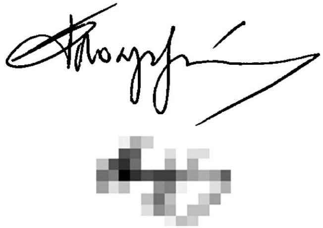
Fig. 4. The grid feature vector of a signature.
