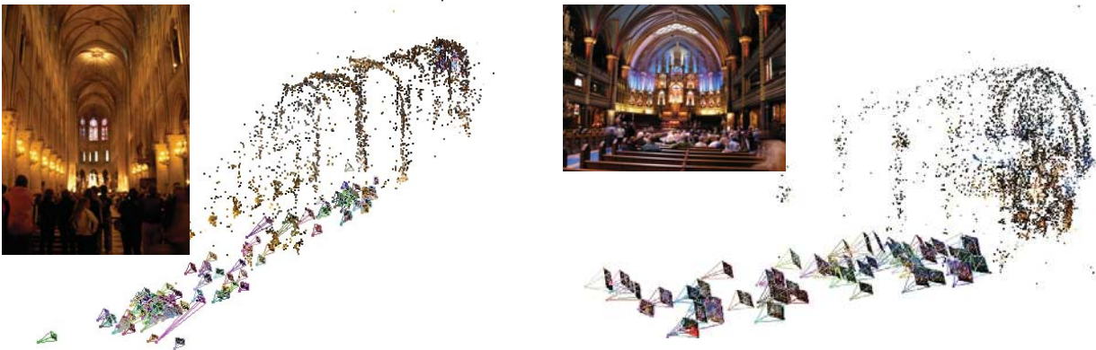
Fig. 16 Two models for different parts of the Notre Dame cathedral interior (118 cameras and 65 cameras, respectively).
